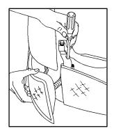
2. Place the tip of a screwdriver through the rectangle hole in the headlamp bracket. Apply pressure to the snap feature (toward the outboard side of the vehicle). Guide the lamp forward.
